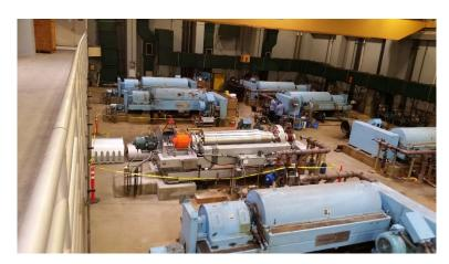
The dewatering centrifuges are part of Area 76, within the Metro Biosolids Center (MBC), a regional biosolids processing facility located adjacent of the City's Miramar Landfill in Kearny Mesa and north of Interstate 52.
